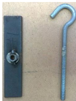
Figure 6: The steel plate and hanger bolt that make up the loading hanger assembly.
