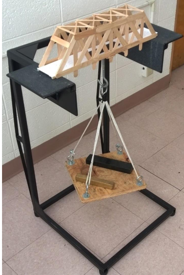
Figure 9: A bridge spanning the two test rig abutments with the loading equipment attached and carrying a gold 2 lb. and black 5 lb. weight. (All weights are now 2 lb. and black).
